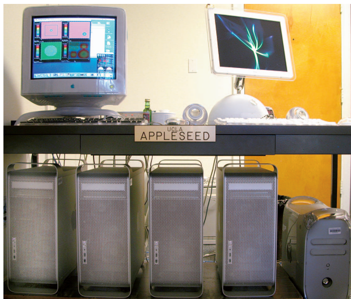
Figure 4. A portion of our Mac cluster. The cluster in the Department of Physics at the University of California, Los Angeles, features a mix of Power Mac G5s and their predecessors. It routinely combines dedicated nodes with desktop machines to perform physics calculations.
