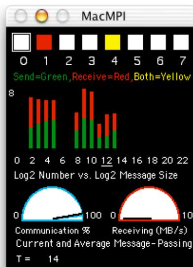
Figure 3. The monitor window of MacMPI, which keeps track of statistics about the execution of the running parallel application.
